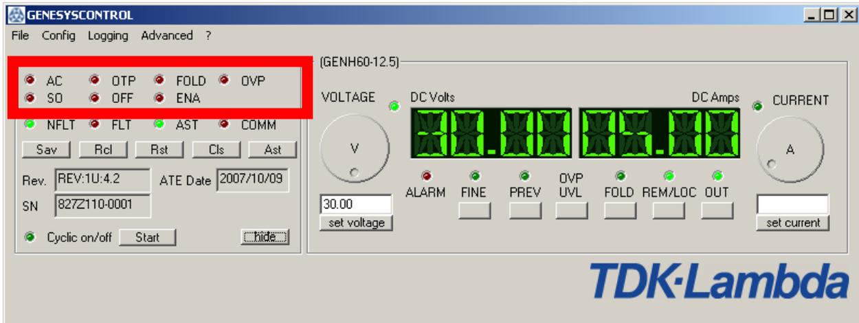
The alarm LEDs display the specific cause for an alarm of the Genesys device. The following alarms can occur:
