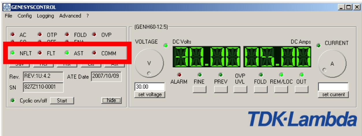
The state LEDs give information about the current state of the Genesys device. There are the following LEDs:
