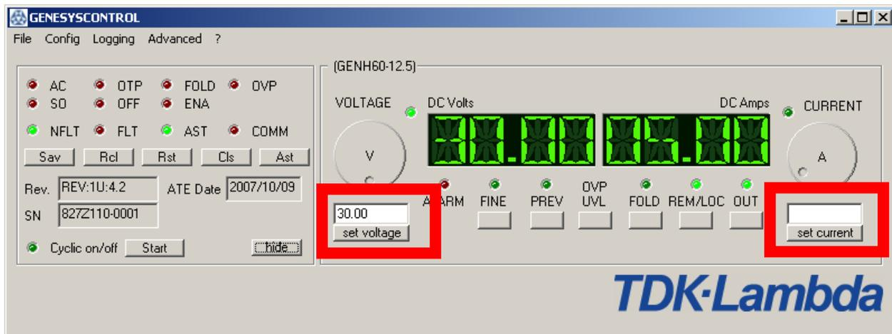
Below the both sliders to control the voltage and the current there are two input fields and two buttons to directly enter any voltage or current. Just enter the value and press the button “set current” or “set voltage” and the current/voltage will be set.
