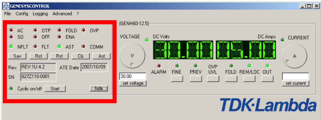
The *Advanced Settings* consist out of four parts: the state LEDs, the alarm LEDs, the command buttons and the info fields. Please see the following sections for more informations about these parts.
