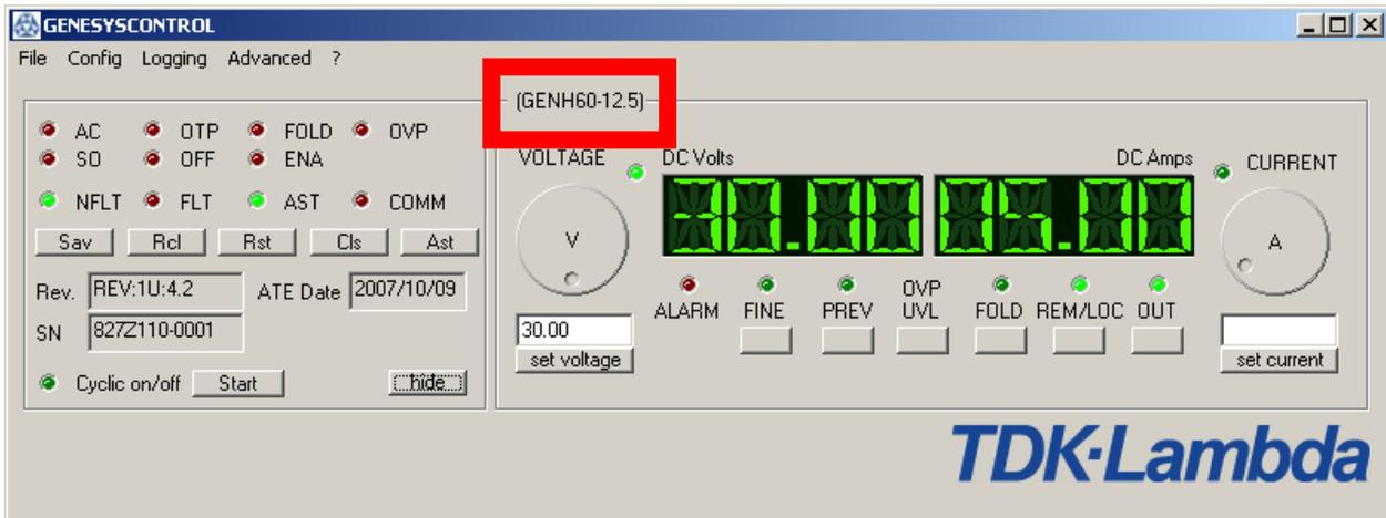
Above the frontpanel you can see the device name and the device type. The device type relies on the Genesys device and the device name can be changed by the user in the *Device configuration*.
