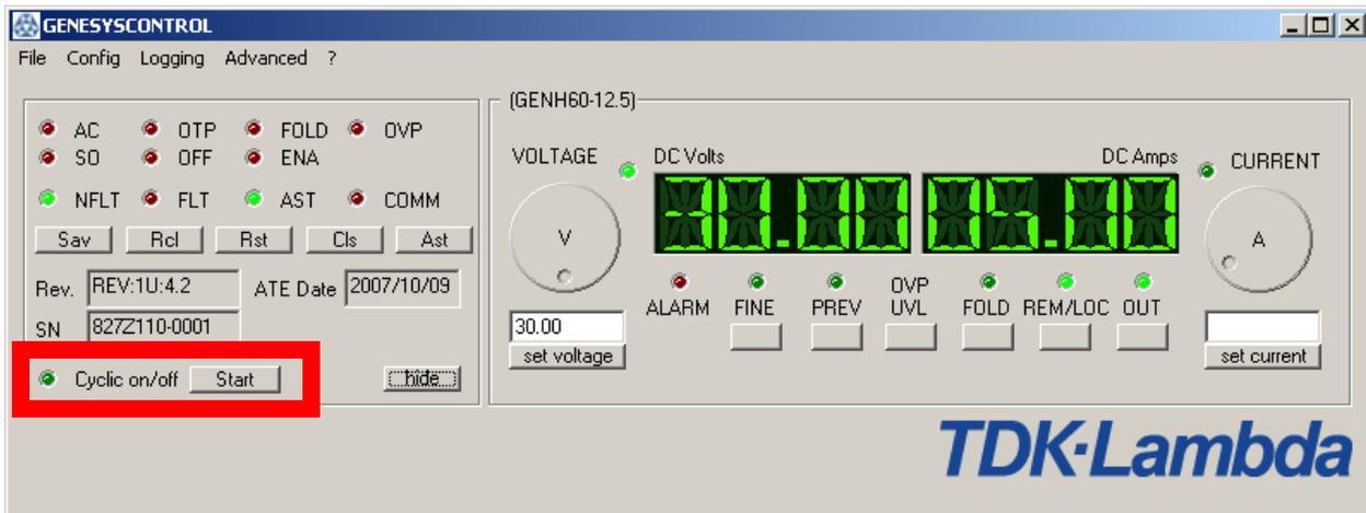
If you click the “Start” button, GenesysControl will display a dialog where you can enter an ON-time and an OFF-time. After pressing again the “Start” button, GenesysControl will switch ON and OFF the selected Genesys device until you stop this function.
