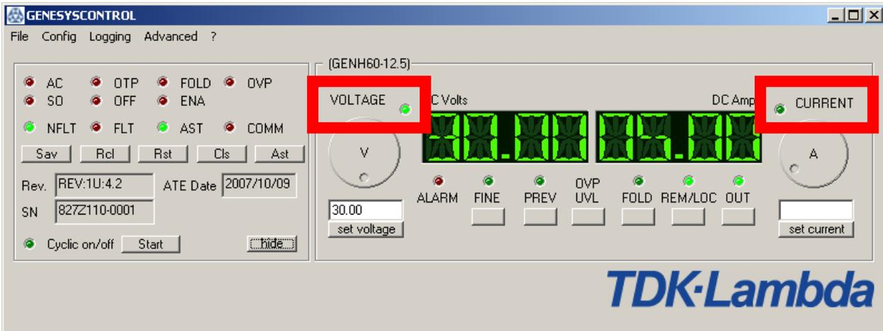
The two LEDs between the sliders and the displays show the output mode of the Genesys device. If the left LED near the voltage slider is on the device is in constant-voltage (cv) mode. If the other LED is on the device is in constant-current (cc) mode.
